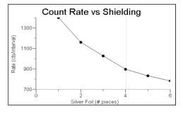
Counts/interval vs. thickness of filter
