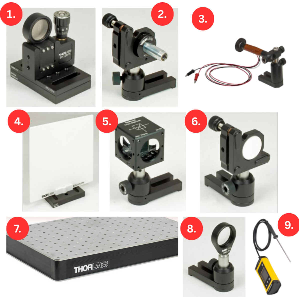
Figure 5: Michelson Interferometer Components
